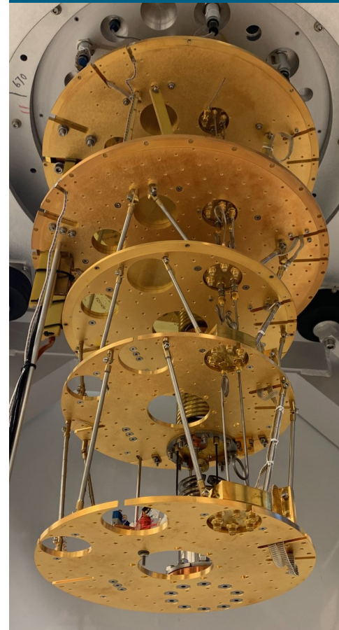
This dilution fridge can achieve temperatures below 10 mK.
