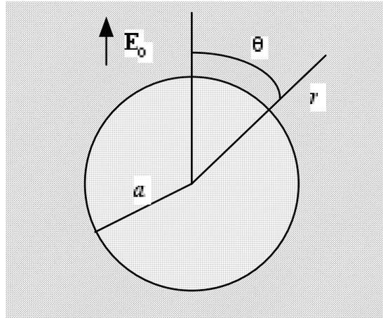
a) Since charges can only accumulate on the inner and outer surface of the insulator, sketch the distribution of charge once equilibrium (for the insulated spherical conductor) and a steady state current (for the external conducting medium) is reached. What is the value of the electric field inside the conducting sphere? What is the value of the electric field far from the conducting sphere?
