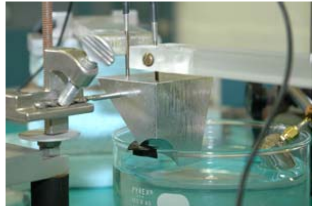
An aluminum block interacts with electronic auto-oscillator circuits via piezoelectric transducers to form a uaser.
